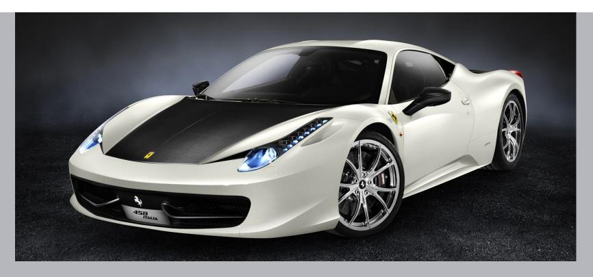
The **weight reduction kit** of 458 Italia is composed by 5 different products that used altogether reduce the vehicle weight of 20 kg as well as highly customize the appearance and the sound of the car. The package can be purchased as a kit, but there are also available the individual components. The carbon of the package is available with a 80 gloss finish. For details on the individual components, please refer to the following pages.
